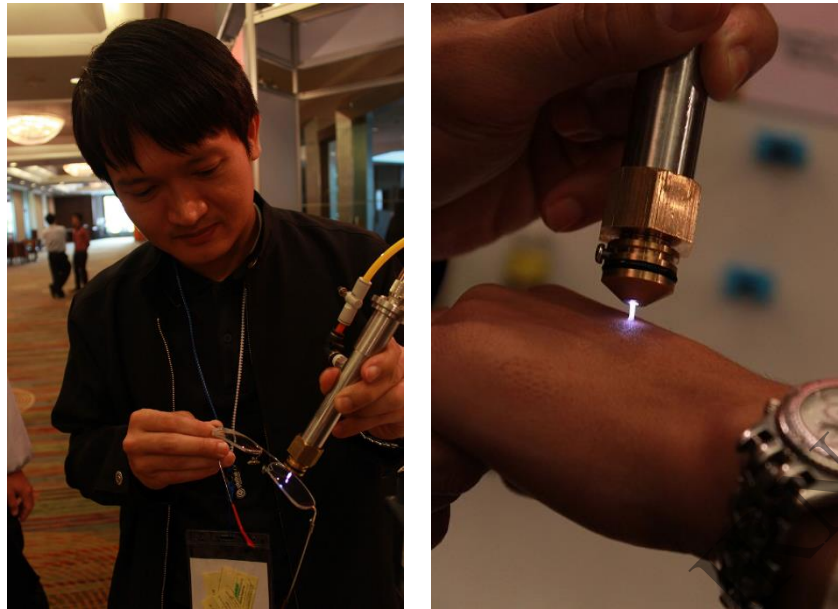
Fig. 2. First prototype of atmospheric pressure plasma jet. Photography by Ruttiya Hong-tong (2009)
